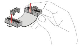
Figure 3–3 ATI CrossFireX Installation
