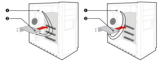
Figure 1–2 Possible Power Connection Locations on the Graphics Card
